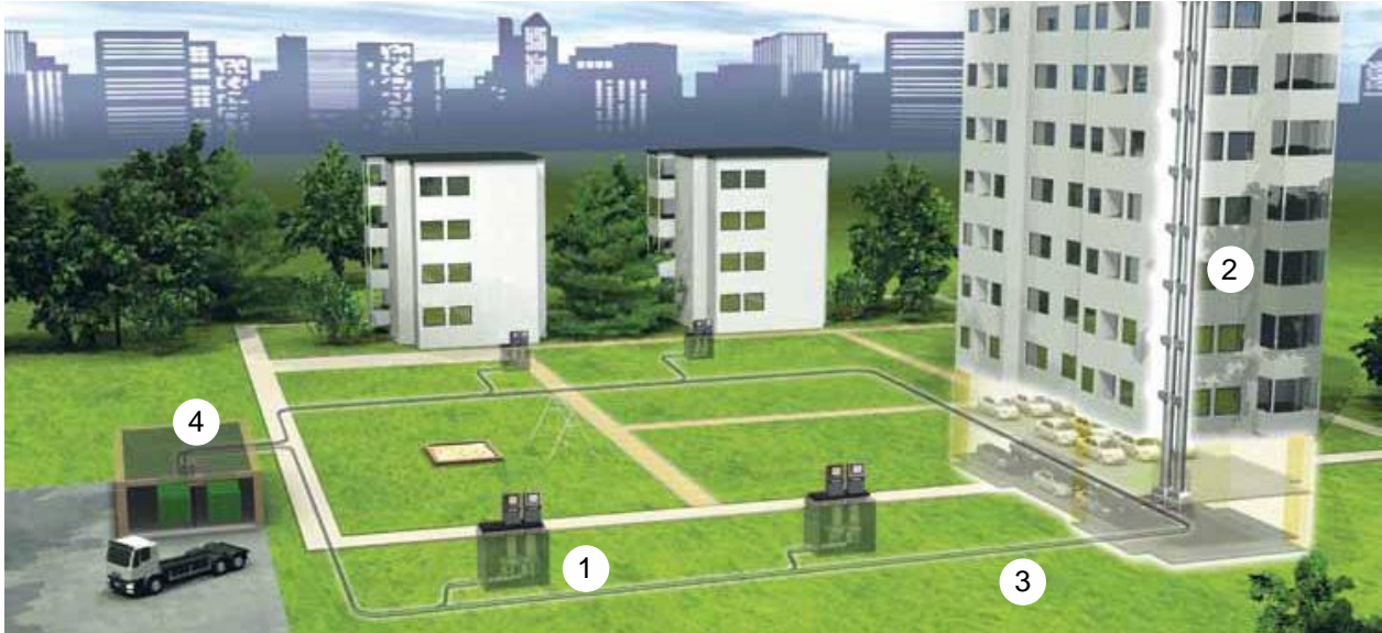
1 Exterior Inlets 2 Interior Inlets 3 Pipeline 4 Collection Terminal
