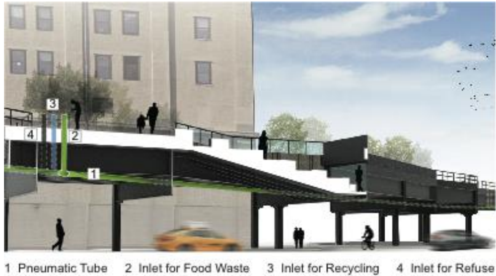
Figure 5. Rendering of Pneumatic Network Along High Line (Colin Curley and ClosedLoops LLC, 2014)
