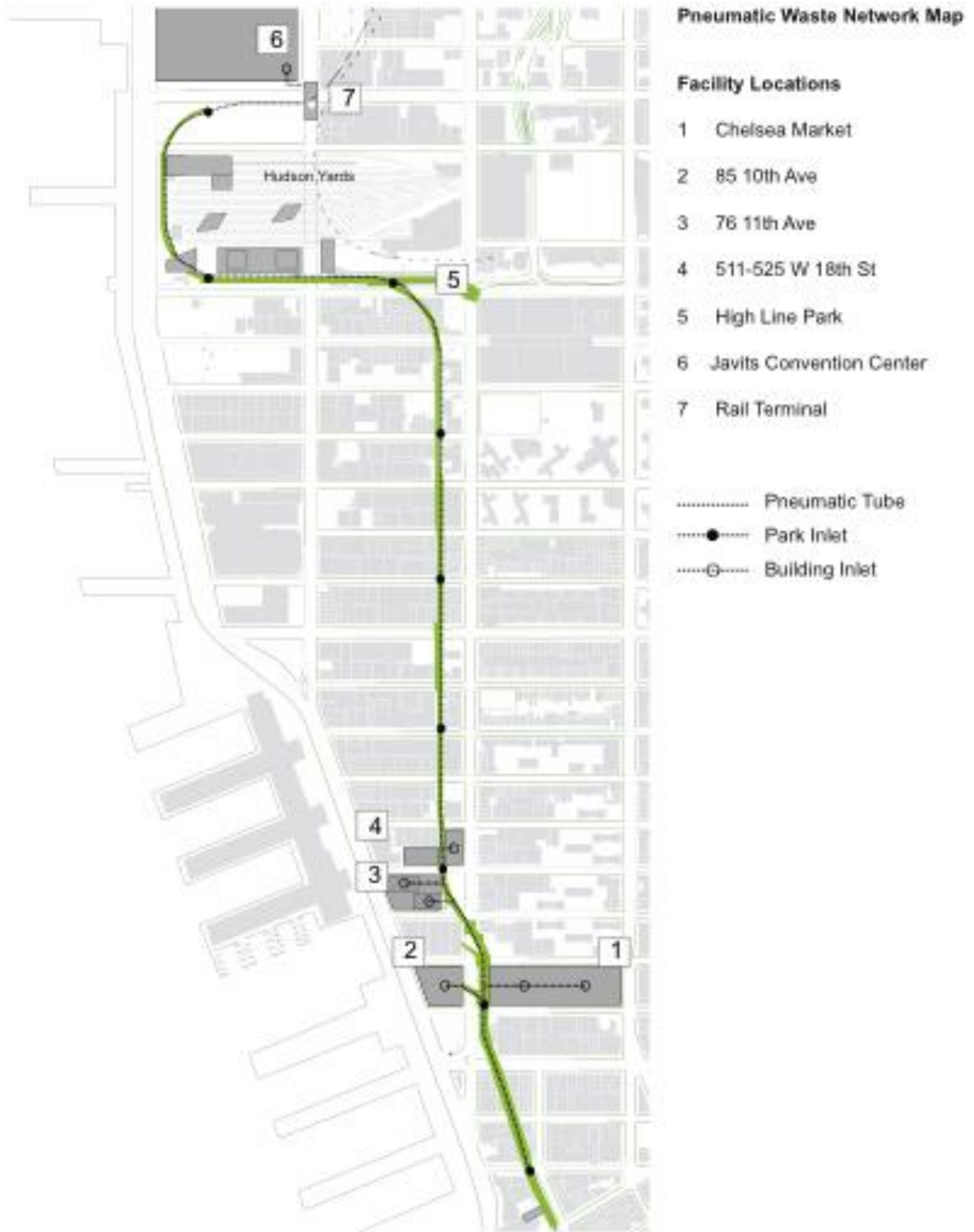
Figure 7. Pneumatic Waste Network
